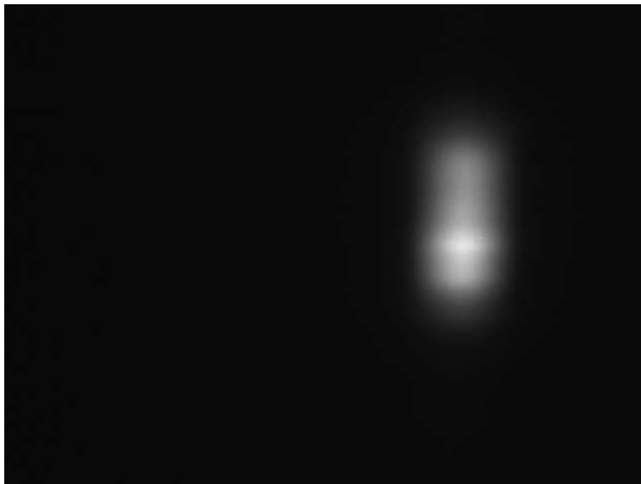
Figure 22: Reference spot of matrix high beam
