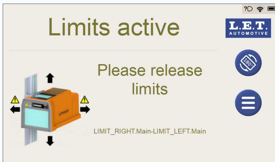
Figure 49: Hardware limit switch active for the horizontal movement
