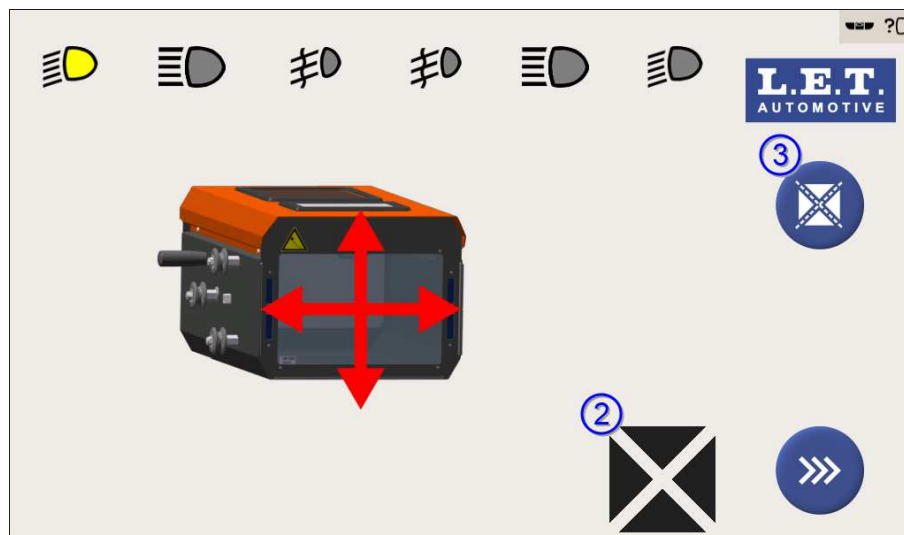
Figure 46: Position Check Arrows on control panel screen
