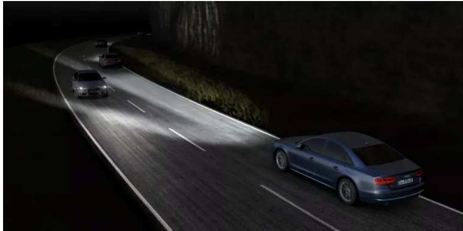
Figure 23: Matrix high beam simulation scene
