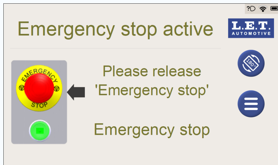
Figure 40: Emergency stop button pressed.
