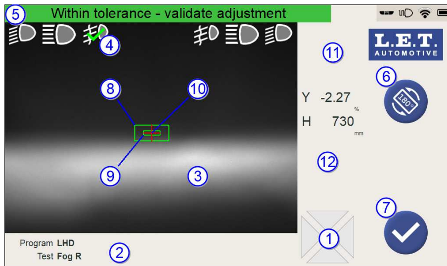
Figure 57: Example of a fog beam
