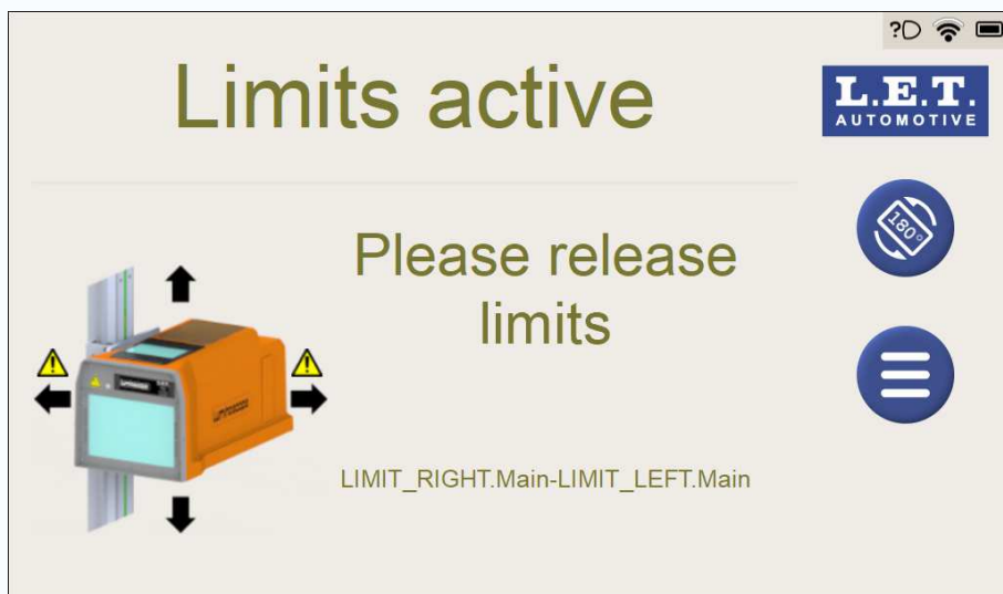
Figure 49: Hardware limit switch active for the horizontal movement
