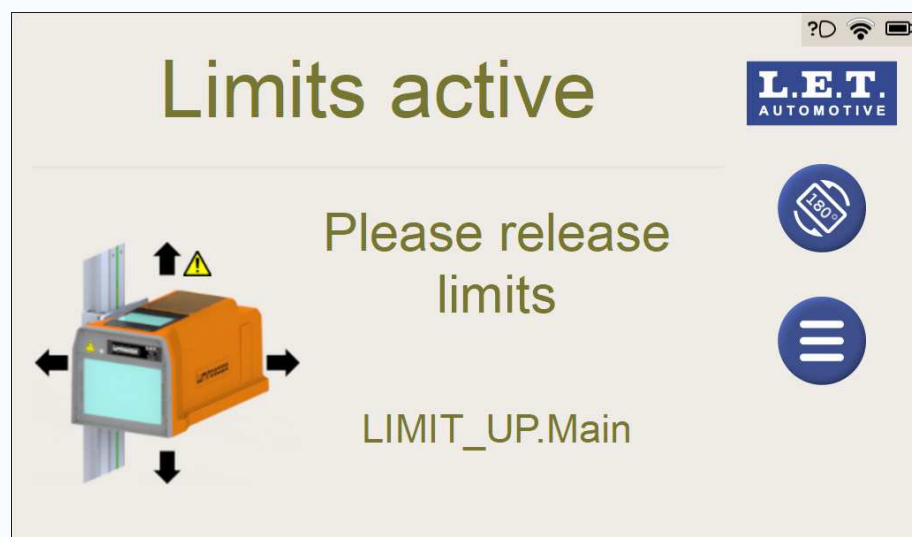
Figure 47: Hardware limit switch active at the highest position for the vertical movement.
