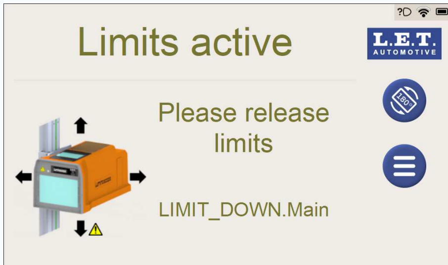
Figure 48: Hardware limit switch active at the lowest position for the vertical movement.
