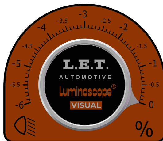
Figure 38: Rotary inclination knob for the low beam inclination
